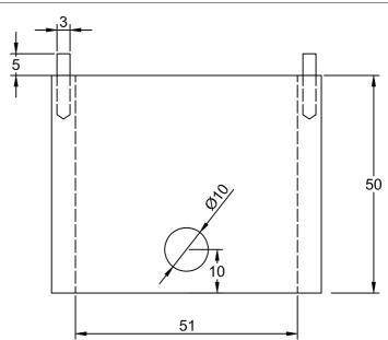
Tool for Group. Use a steel pipe with outer diameter 62 and inner diameter 51. For the 3mm pins you can use old drills or Sellock Roll Pins. The 10mm hole is for a extention of a ratchet, so you can open the thread.
