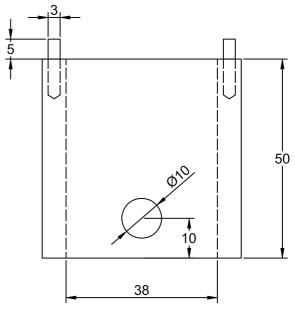
Tool for Glas. Use a steel pipe with outer diameter 50 and inner diameter 38. For the 3mm pins you can use old drills or Sellock Roll Pins. The 10mm hole is for a extention of a ratchet, so you can open the thread.
